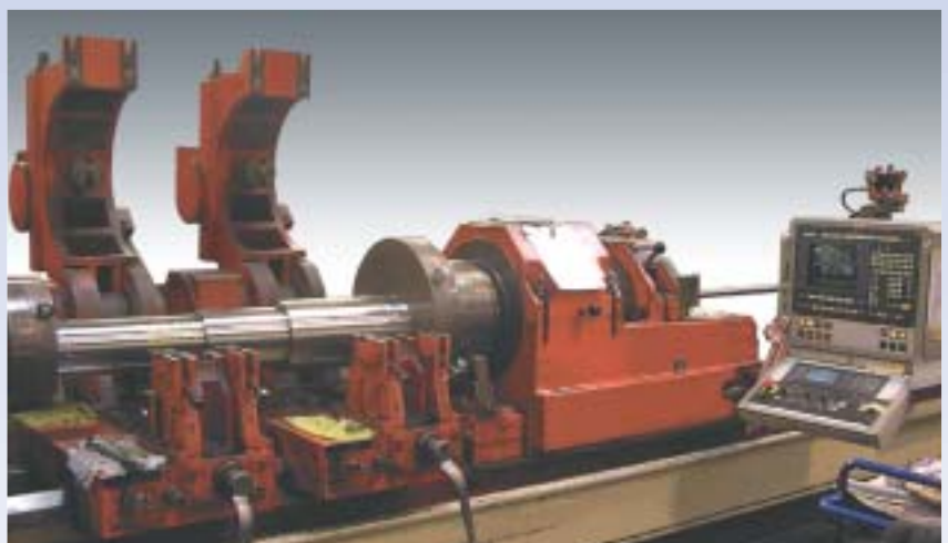
Deep hole drilling
